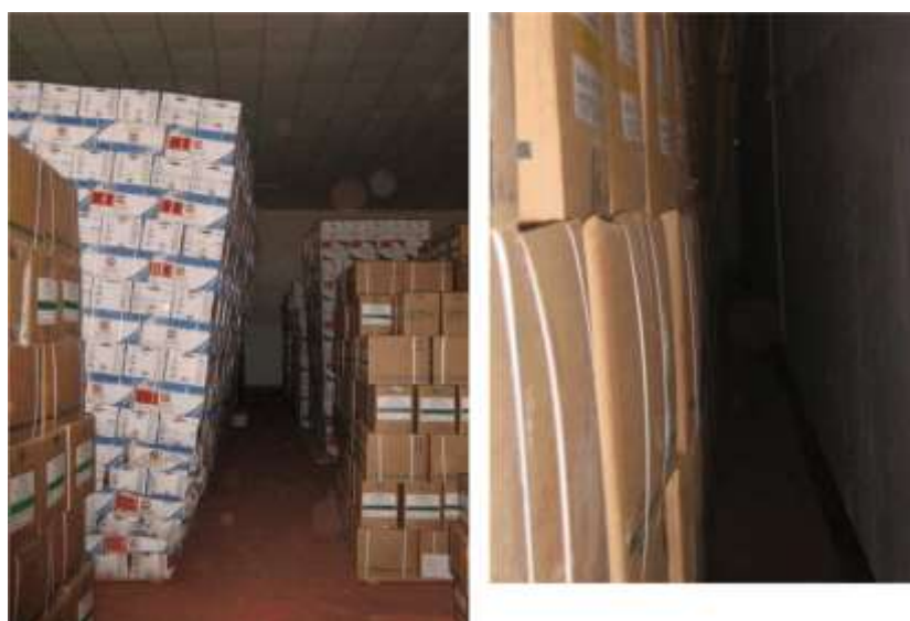
1. Overloaded block stack with some damaged cartons
