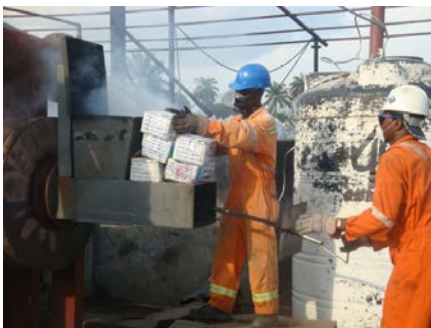
Workers at the BOSKEL Nigeria facility add expired ARVs to an incinerator.
