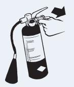
Pull the pin at the top of the extinguisher.
