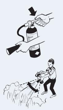
Squeeze the handle to discharge the extinguisher (stand approximately 2.5 m [8 ft] away).
